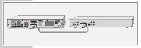
1 Connect the »EURO AV2 → DECODER« socket on the HDD DVD recorder to the corresponding socket on the video recorder, DVD player or set-top box using a standard EURO-AV (SCART) cable.
